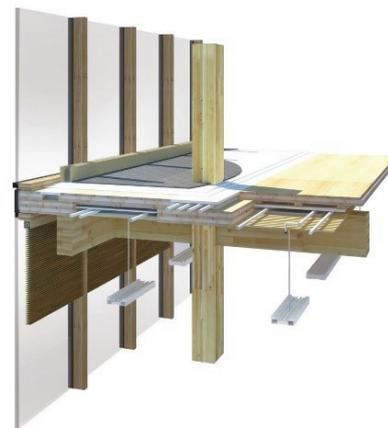
Рис. 8. Схема конструктивной системы CREE. Источник: <https://www.archdaily.com/630264/wood-innovation-design-centre-michael-green-architecture/5552153be58ece92c700026f-wood-innovation-design-centre-michael-green-architecture-detail>
